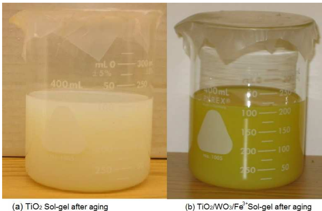
Figure 4.5 Prepared Template \text{TiO}_2 Based Sol-gel Samples. (a) Template \text{TiO}_2 Sol-Gel Sample after Aging; (b) Template \text{TiO}_2/\text{WO}_3/\text{Fe}^{3+} Sol-gel Sample after Aging
